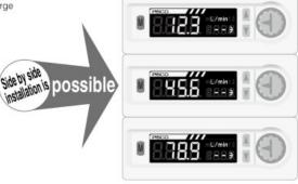
Dual display / 2 color indication feature. Introduction of main and sub display improve operability. Additionally, 2 colors indication makes easy cognition of error.
